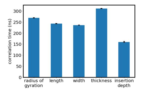
Supplementary Figure 8. Correlation times of the fusion peptide shape properties during MARTINI coarse-grained simulation of an equilibrated fusion peptide bound to a membrane.
